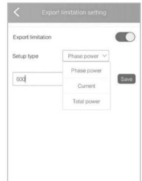
Figure 6.4 Power limit/Current limit setting
