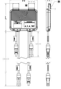
\*Clips can be removed for rack mounting
